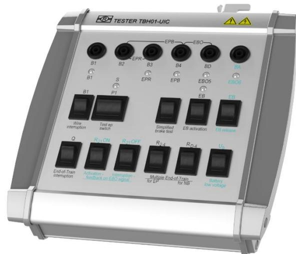
Direct on the front side of the device there are placed 6 sockets for lines No. 1,2,3,4,D,A of the 9-core brake cable for direct Voltage check between the lines according to UIC541-5.
